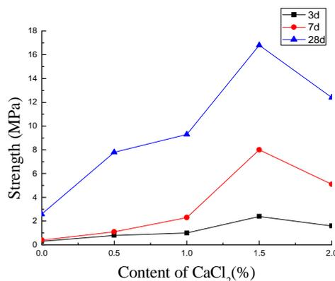
**Fig.2 Effect of  $\text{CaCl}_2$  on compressive strength of steel slag-slag powder**
