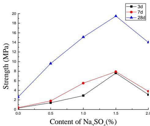
**Fig.3 Effect of sodium sulfate on compressive strength of steel slag-slag powder**
