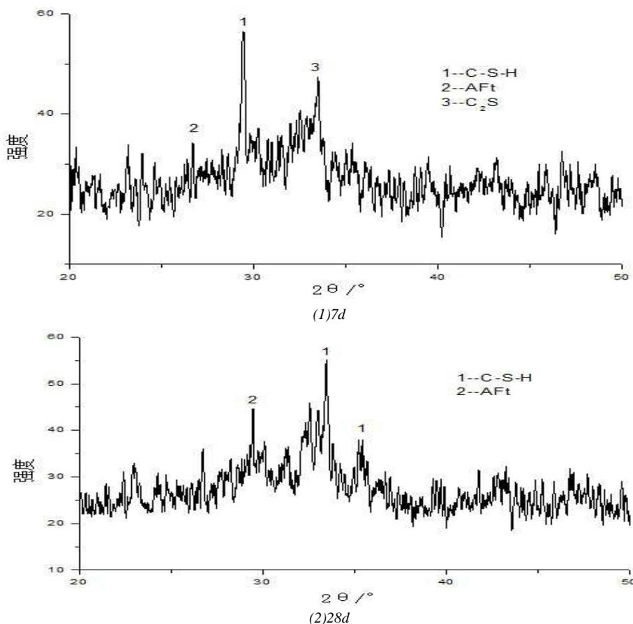
Fig.4 XRD patterns of specimen with 1.5% sodium sulfate of complex accelerator at 7d and 28d
