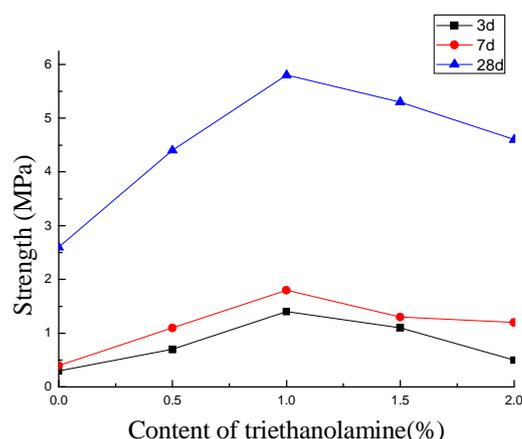
Fig.1 Effect of triethanolamine on compressive strength of steel slag-slag powder
