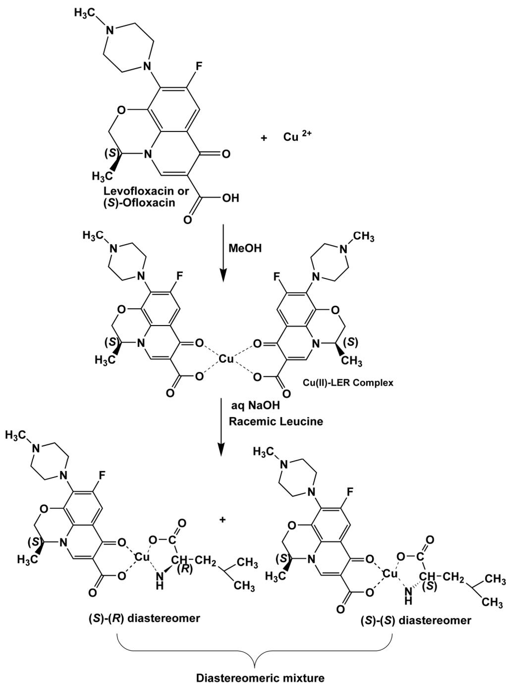
**Fig. 3:** Separation mechanism for amino acids using Levofloxacin as ligand exchange reagent
