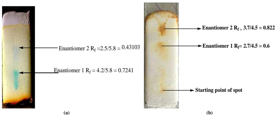
Fig. 2. Actual photographs of TLC for the enantioseparation of (a) Tryptophan and (b) DL-2-amino butyric acid
