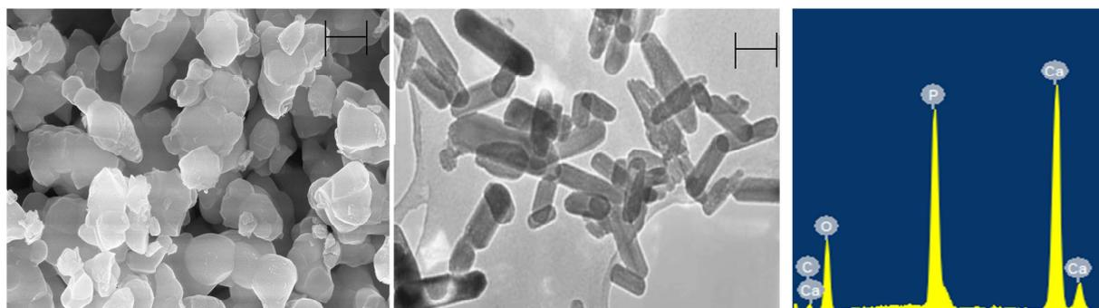
Figure 4 : FESEM of HAp synthesized Without and with CTAB & EDAX
