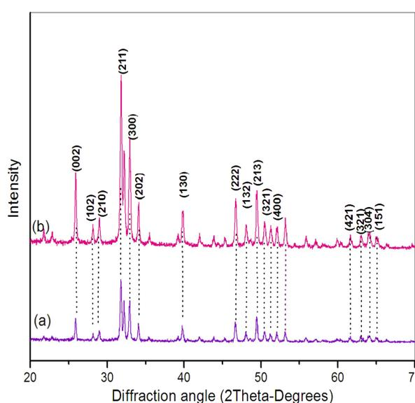
Figure 2: XRD pattern of (a) Pure HAP (b) With CTAB
