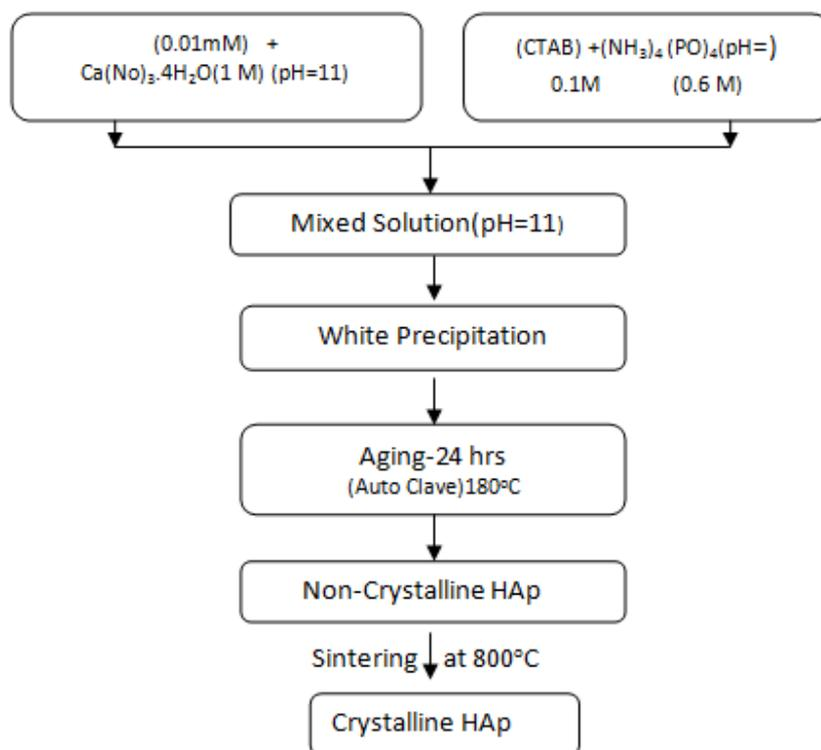
Figure 1: Flow chart of synthesis of HAp
