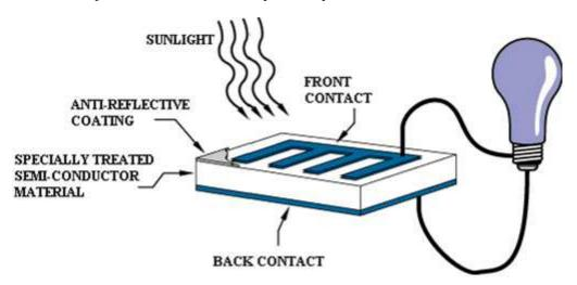
Fig.2. Generation of electricity by the help of sunlight when it incident on the semiconductor material
