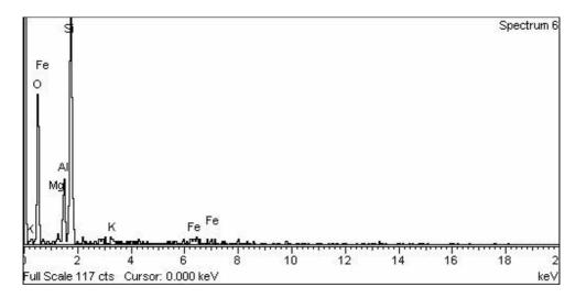
Fig. 2. EDX analysis of raw bentonite
