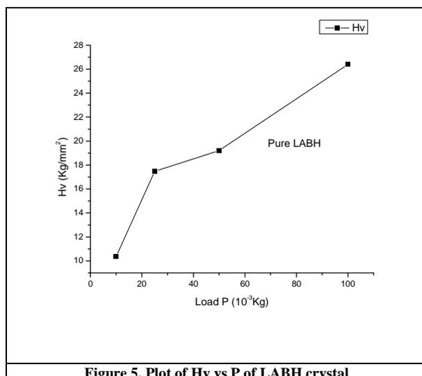
Figure 5. Plot of Hv vs P of LABH crystal
