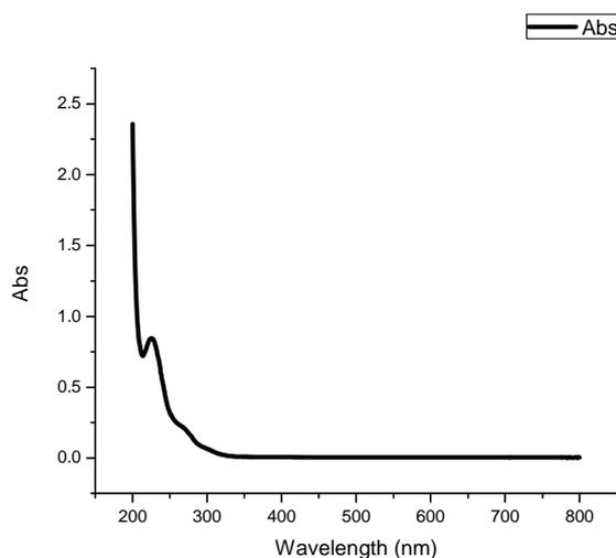
**Figure 3. Optical absorption spectrum of LABH crystal**
