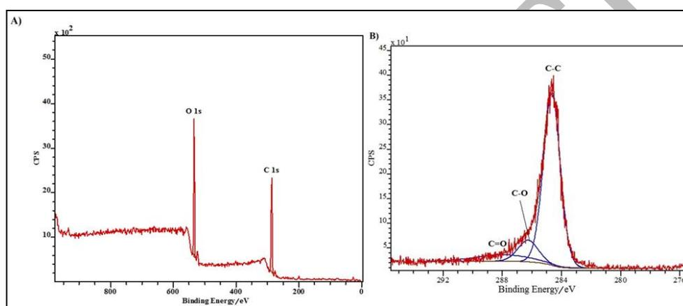
Figure 4: The XPS (a) and C1s (b) spectra of the as-obtained CDs
