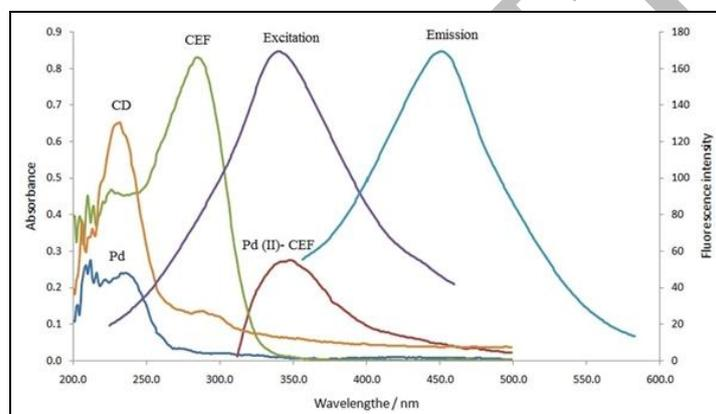
Figure 1: UV-Vis spectrum of CEF, Pd, Pd(II)-CEF complex and CDs with normalized fluorescence spectrum of CDs
