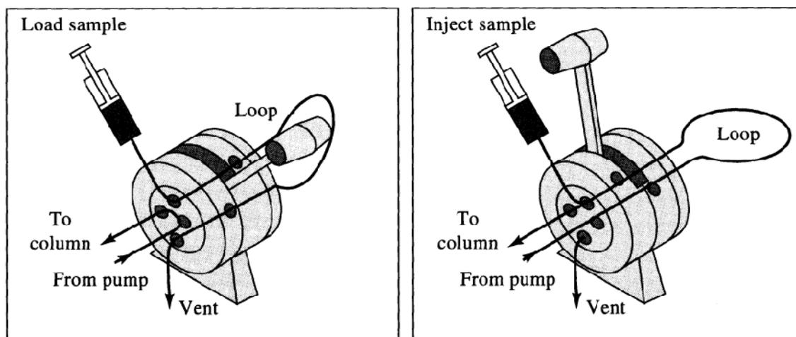
**Fig 4: An injection valve**
