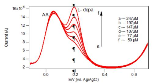
Figure 10 DPV of 5mM AA at PEDOT-PSS GCE in the presence of different concentration of L- dopa: (a) 50.0, (b) 77.0, (c) 107.0 (d)
