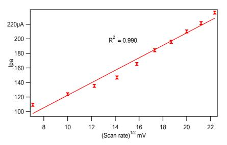
Figure 7 Square root of scan rate vs. anodic peak current of L-dopa in PEDOT-PSS modified GCE
