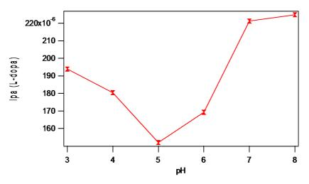
Figure 8 Ipa of L-dopa in different pH (from 3.0 to 8.0) at PEDOT -PSS GCE
