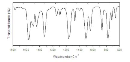
Figure 3 ATR-IR spectra of EDOT monomer
