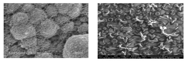
Figure 2 SEM image of (a) PEDOT, (b) PEDOT-PSS
