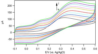
Figure 6 CV of the 5mM L-dopa in PBS (pH 7.0) at PEDOT-PSS modified GCE with different scan rates (a-j: 50, 100, 150, 200, 250, 300, 350, 400, 450 and 500 mVs<sup>-1</sup>)
