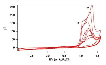
Figure 1 Cyclic voltammogram of PEDOT-PSS
