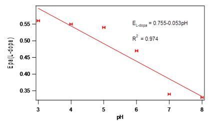
Figure 9 Plot of Epa vs different pH for 5mM L-dopa in PEDOT-PSS modified GCE
