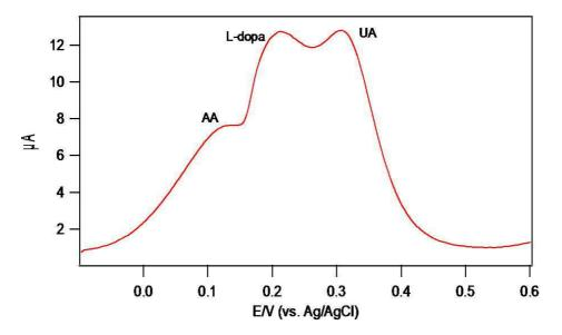
Figure 12 DPV of 1mM L-dopa, AA and UA in PEDOT-PSS GCE
