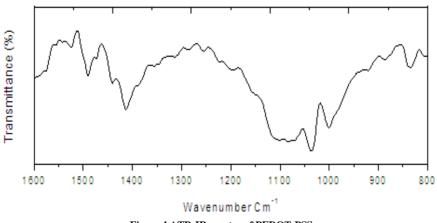
Figure 4 ATR-IR spectra of PEDOT-PSS
