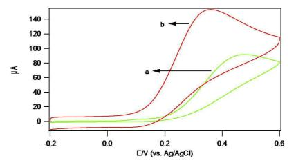
Figure 5 Cyclic voltammogram of 5mM L-dopa, (a) bare GCE (b) PEDOT-PSS GCE at pH 7.0
