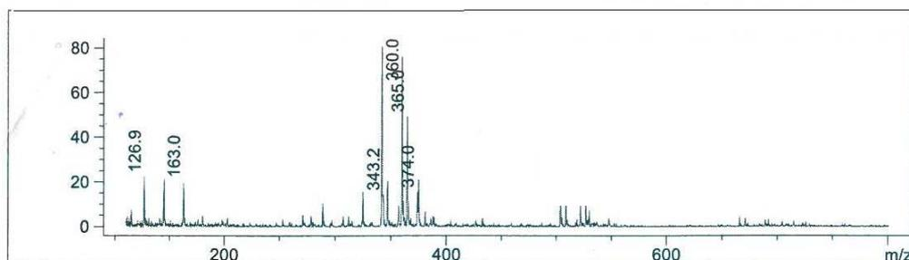
**Figure 19. MS Report for the Separated Fraction3 (Time 0.507 : 0.600)**
