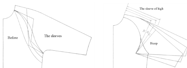
Fig.1 Change in Armhole Arc of Raglan Sleeve & Width of Raglan Sleeve
