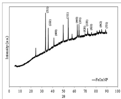
Fig. 3: XRD pattern of Iron oxide nanoparticles
