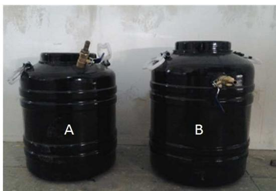
Fig 1: Portable food waste digesters
