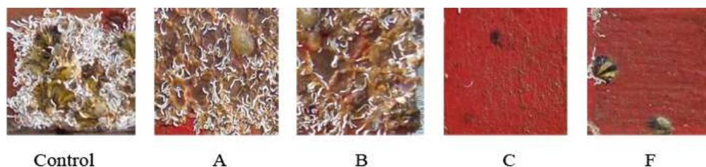
Figure 1 Anti-biofouling performance of micro/nano coatings after an exposure to marine environment for 11 months
