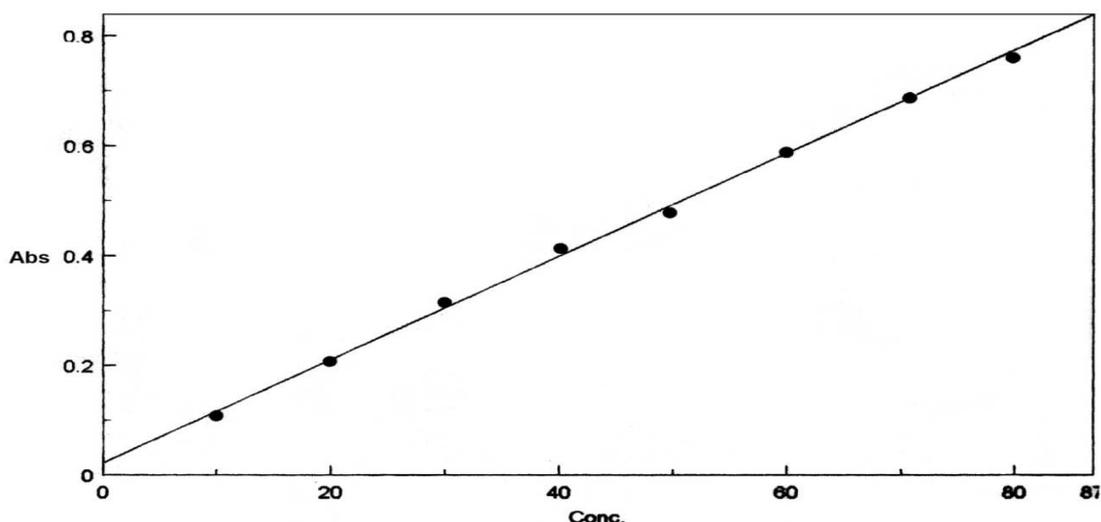
**Figure 2: Calibration graph of Voglibose 282 nm**
