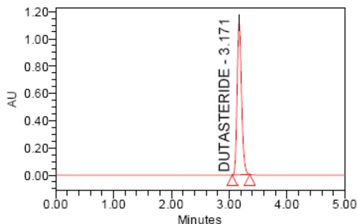
Figure 4: Chromatogram of standard dutasteride sample (40 µg/ml)
