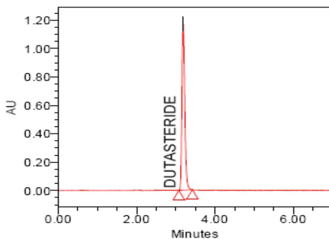
Figure 10: Chromatogram of dutasteride after photolytic degradation
