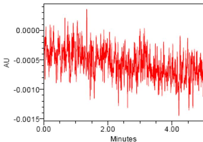
Figure 2: Chromatogram of mobile phase blank
