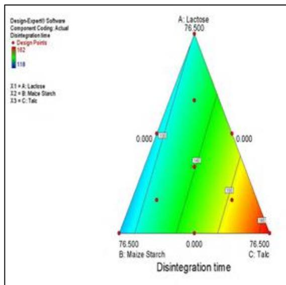
Figure 5: Response graph for disintegration time
