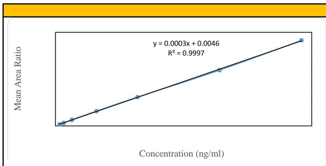
Figure 7: The plot of linearity for mean six calibration curves
