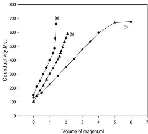
Figure.4: Conductimetric determination of 21.25 mg AlFCl using  $10^{-2}$  M STA (a), PTA (b), NaTPB (c)
