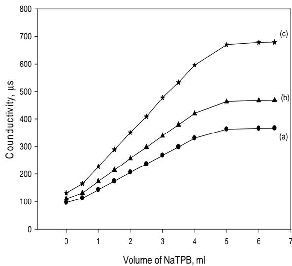
Figure.3: Effect of dilution on the end point of the conductimetric titration of 21.25 mg AlFCl with  $10^{-2}$  M NaTPB in total volume 50 ml (a),75 ml (b),100 ml (c)
