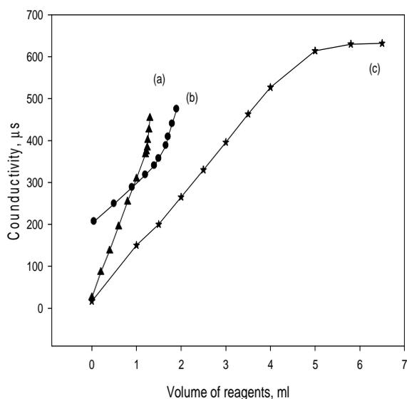
Figure 5: Conductimetric determination of 22.25 mg TamCl using  $10^{-2}$  M STA (a), PTA (b), NaTPB (c)
