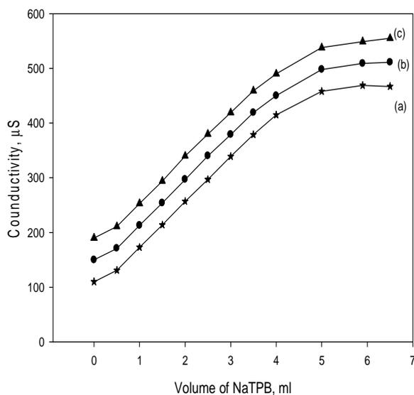
Figure 2: Effect of temperature on the end point of the conductimetric titration of 21.25 mg of AlfCl with  $10^{-2}$  M NaTPB at 25 (a), 35 (b), 50°C (c)
