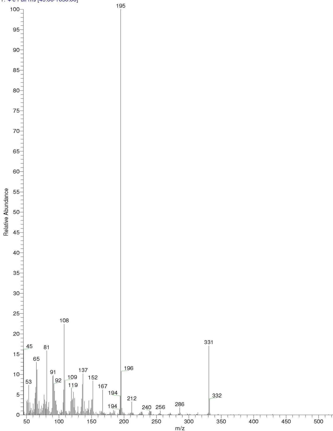
Figure 2: Mass Spectrometry of Compound M1: MS (amu) 331(M<sup>+</sup>); 195 (C<sub>10</sub>H<sub>11</sub>O<sub>4</sub>)
