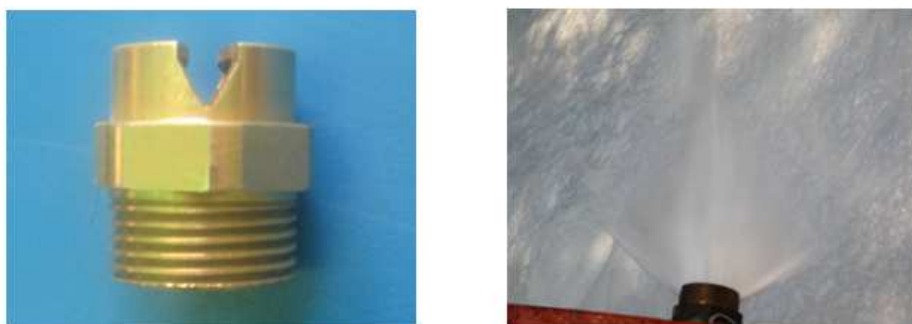
Fig. 11. Special foam nozzle and its injection effect
