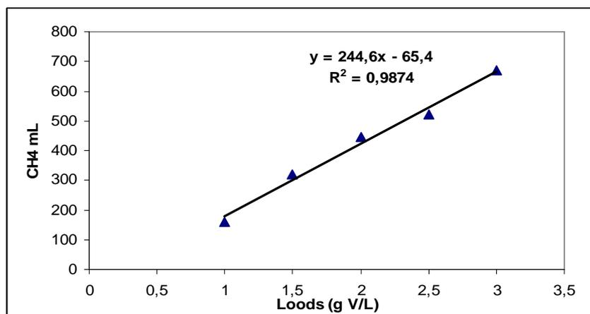
Figure 2: Regression between changes in CH<sub>4</sub> concentration and load
