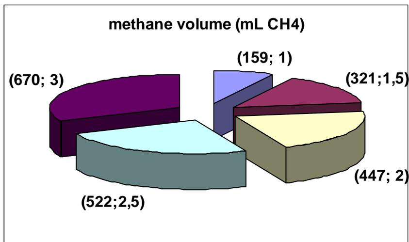
Figure 1: The methane production during the anaerobic digestion of sewage sludge for different loads (from 1.00g to 3.00g SV)
