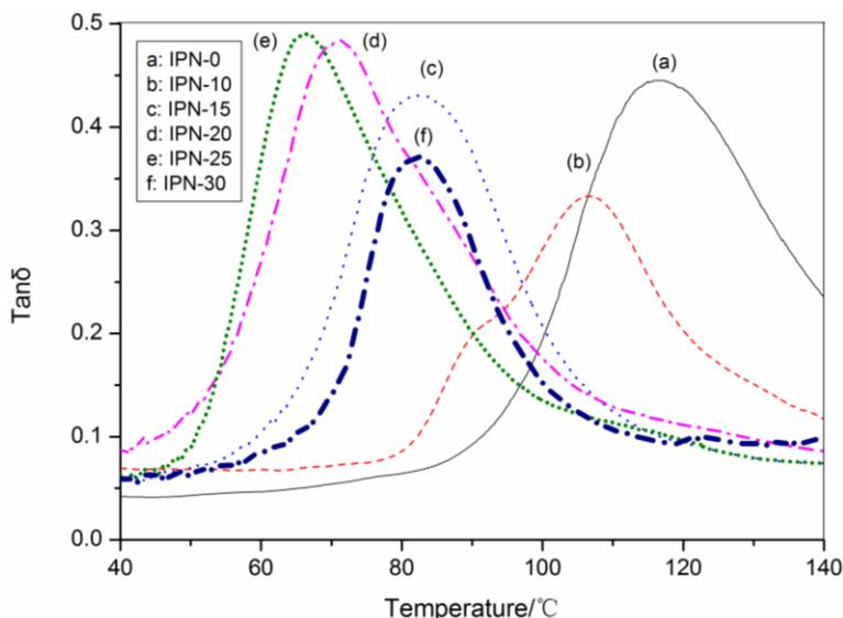
Figure 5: Dependence of  $\tan\delta$  versus temperature of different IPNs
