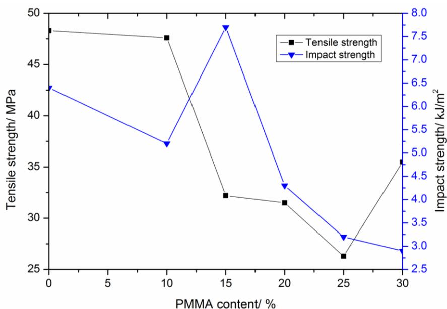
Figure 2: Mechanical properties of PMMA/EP IPNs
