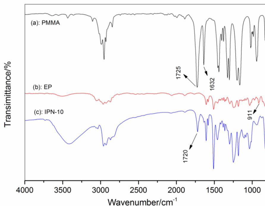
Figure 1: FT-IR spectra of (a) PMMA, (b) EP and (c) IPN-10
