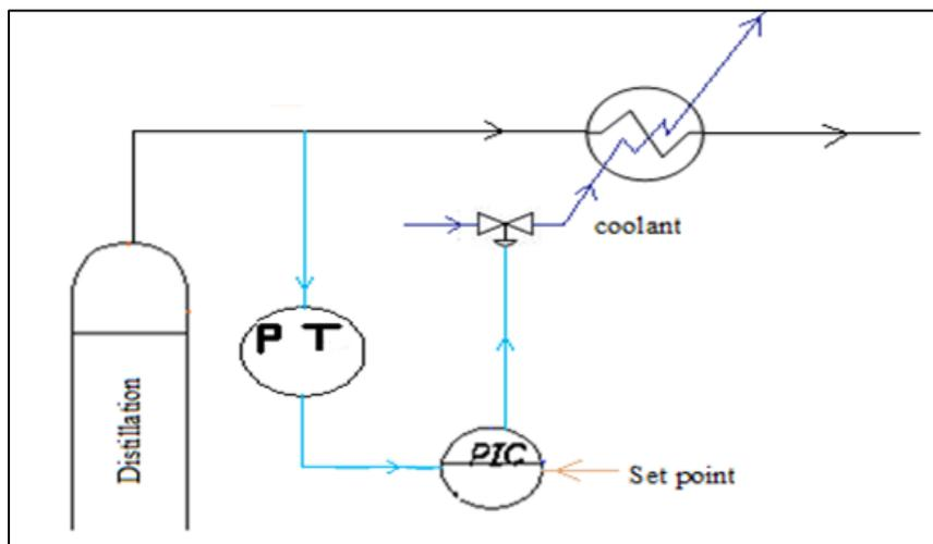
**Figure 2: Process control diagram for fractionator overhead pressure**
