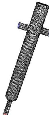
Figure 3 Meshing of the nozzle studied by CFD
