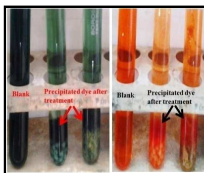
Figure 2 Fabric dye precipitation after treatment with Chara beads and Chara sp. (FD2 and FD3)
