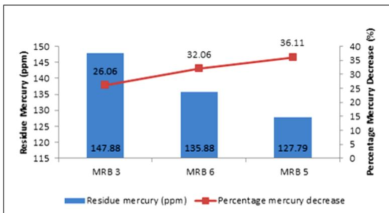
**Figure 3: Residu mercury and percentage mercury decrease on day thirty after incubation using superior mercury resistant bacteria isolate *ex-situ* with simple closed bioreactor**
