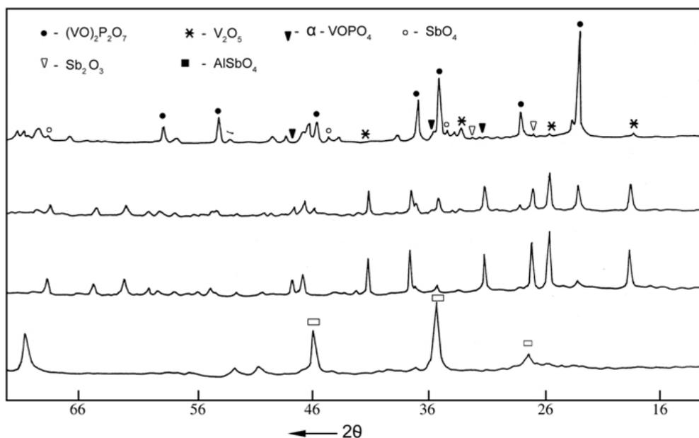
FIG. 1 - X-Ray Diffraction Patterns of Sb-VPO Catalysts
