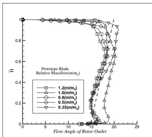
c) Forward-swept rotor cascade outlet flow angle
