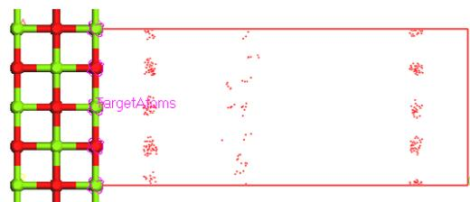
Figure 6 Profile of SO<sub>3</sub> adsorption on MgO(200) at 973 K
