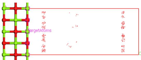
Figure 5 Profile of SO<sub>2</sub> adsorption on MgO(200) at 973 K
