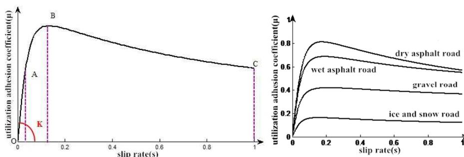
Fig.1 characteristics of  $\mu$  and s Fig.2  $\mu$ -s curve of different road conditions
