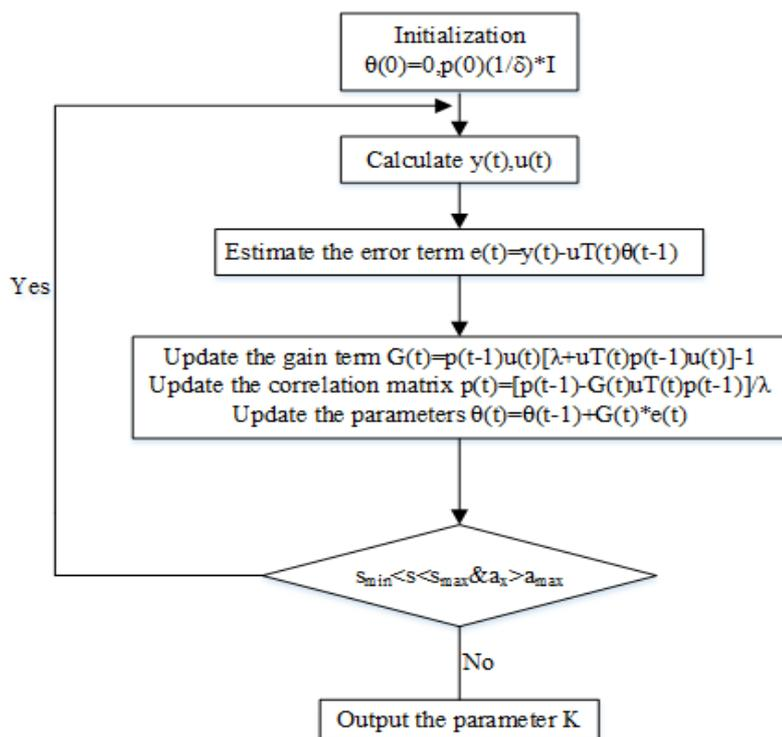
Fig.5 Flow chart of parameter K identification
