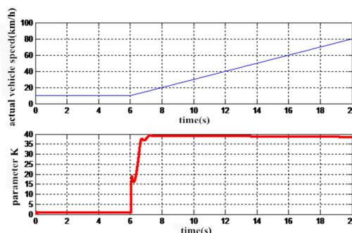
Fig.7 The curve of actual vehicle speed and parameter K on the wet asphalt road surface
