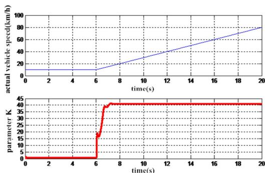
Fig.6 The curve of actual vehicle speed and parameter K on the dry asphalt road surface
