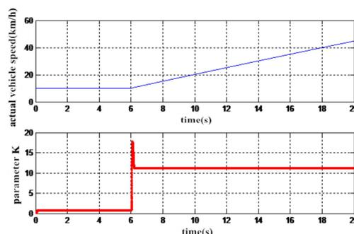
Fig.9 The curve of actual vehicle speed and parameter K on the ice and snow road surface
