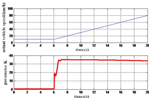
Fig.8 The curve of actual vehicle speed and parameter K on the gravel road surface
