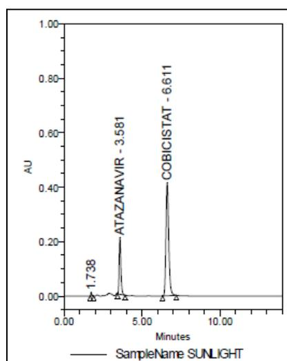
Figure 12: Chromatogram of sunlight stressed degradation of drug product
