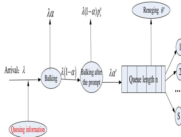
Figure 1. The service flowchart of a call center with delay information
