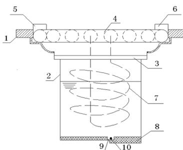
Fig.1 the dimensional sketch of floor drain
